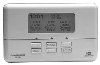
The ChannelPlus family of electronic programmers offer a range of advanced features coupled with simplified 'menu driven' programming all designed to help save energy. The Horstmann ChannelPlus H37XL series 2 is designed to give independent time control over 3 channels of heating or hot water on a 7 day weekly programme. Each channel offers up to 3 programmed On/Off operations per day for each day of the week.
