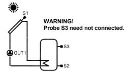
N° 2: Solar heating installation with 1 tank and additional thermostatic heating.
