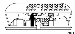
5 Fix the plate to the wall, using the two screw seats with centre distances of 60 mm or 85 mm (use the supplied wall plugs and/ or screws). Pass the wires through the rectangular openings.
