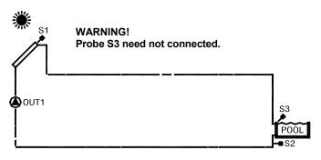
N° 4: Solar heating installation with 1 tank, direct integration by means of valve logic.
