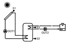
N° 3: Pool solar heating installation.
