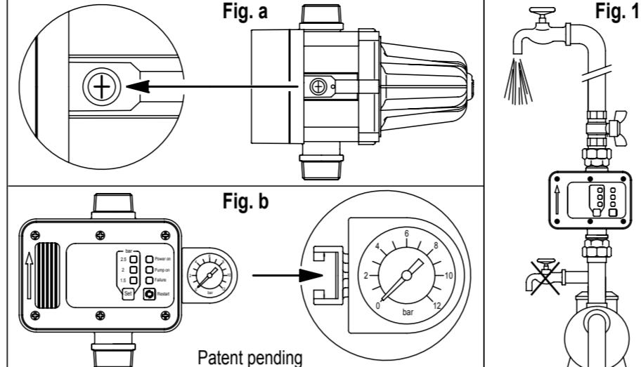
**Device for control and protection of the electric pump****GB ORIGINAL OPERATING INSTRUCTIONS**
