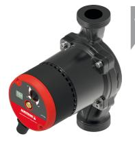
TECHNICAL DATA up to  $4.4 \text{ m}^3/\text{h}$ Rate of flow: Pressure head: 4 m/6 m/8 m Control range: Media temperature: +2 °C to +110 °C Installation length: 130 and 180 mm Threaded connection:  $1^{1}\!\!\!/_{2}^{\prime\prime}$  and  $2^{\prime\prime}$ Protection class: IP 42 Insulation class: PN 10 Nominal pressure: Control: EEI:
