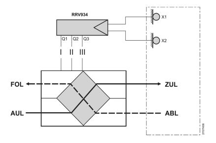
Q1 - Q3 3-stage step selector of ventilation plant Air quality sensor, DC 0...10 V X1 Humidity sensor DC 0...10 V
