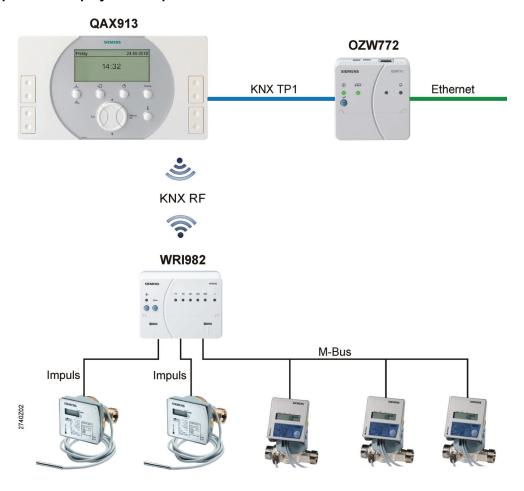
Integrate the consumption data interface WRI982 to display energy consumption on the central apartment unit and send it to a service provider via web server OZW772.
